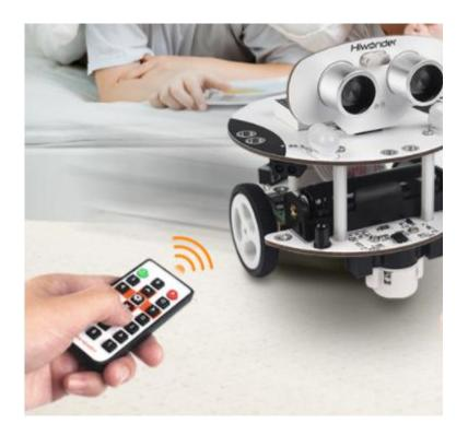
When we press button 2 on the remote controller. Qbot will move forward, and if we press button 8, it will move backward, and press 4 and 6 can let Qbot turn left and right respectively
